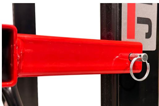
Figure 6-8: Remove Leg Storage Pins
