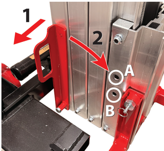
Figure 7-5: Engaging Mast Locking Arm
