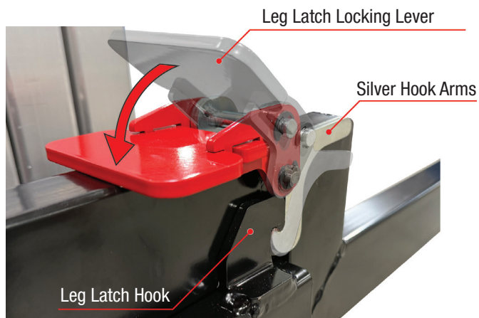
Figure 6-10: Locking Legs In Place
