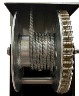
Figure 4-23: Cable Wrapped Tightly and Evenly
