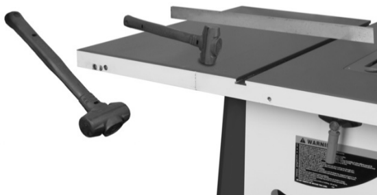
Figure 6-5: leveling extension wings, method
