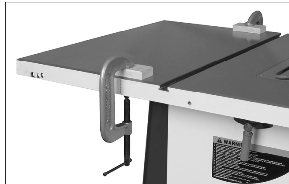
Figure 6-6: leveling extension wings, method 2
