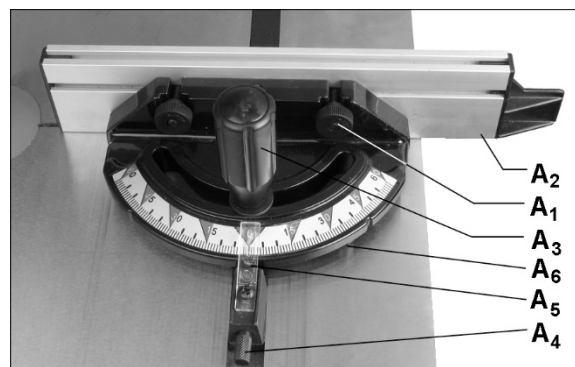
Figure 7-2: Miter Gauge Adjustments
