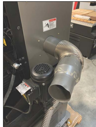
Figure 7-1: Connecting Dust Collection Hose to Dust Hood Outlet
