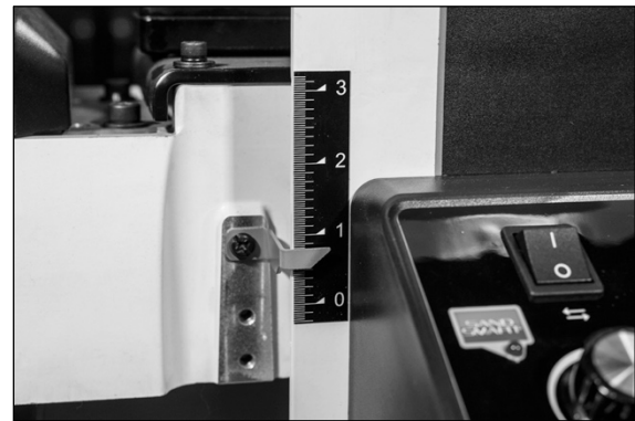
Figure 8-1: Depth Scale Adjustment
