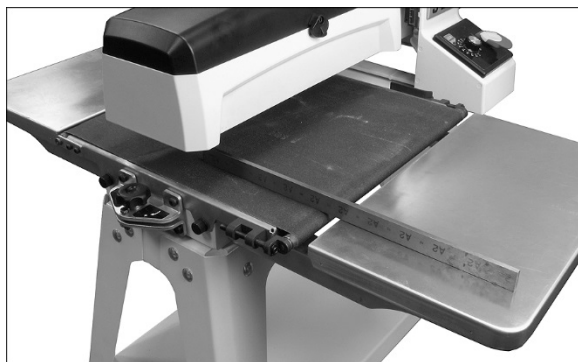
Figure 6-4: Extension Table Alignment
