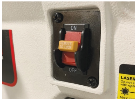
Figure 4-1: Main Power Switch
