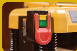
Improved Large E-Stop Enhanced safety. Faster shutdown.
