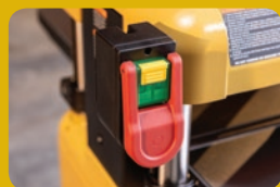
Improved Large E-Stop Enhanced safety. Faster shutdown.
