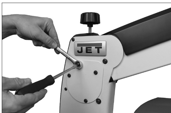
Figure 24: tightening arm lift
