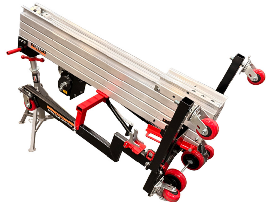
Figure 4-3: Material Lift Tilted and Stabilized
