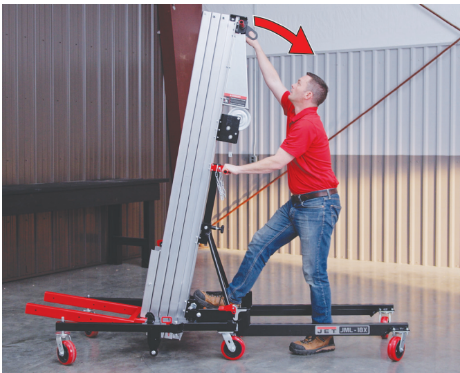
Figure 7-14: Lowering Mast Assembly
