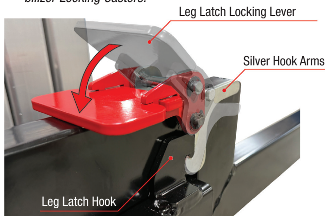
Figure 6-3: Locking Legs In Place
