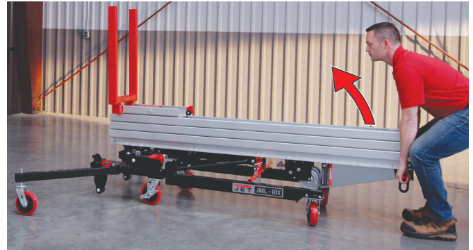
Figure 6-7: Lifting Mast to Vertical Position
