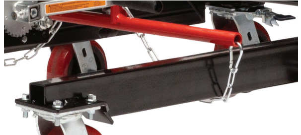
Figure 6-6: Removing Storage Chains
