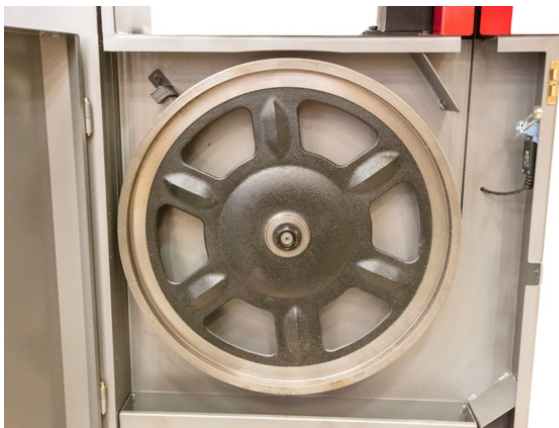
Figure 9-5 Lower Wheel Housing
