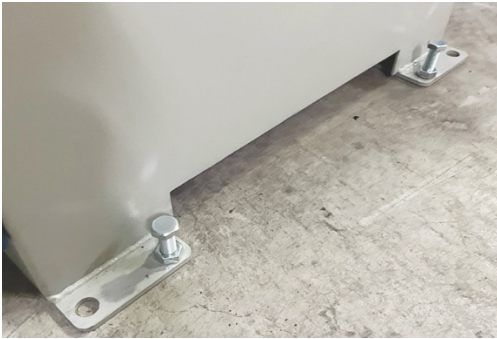
Figure 7-1 Leveling Bolts and Nuts
