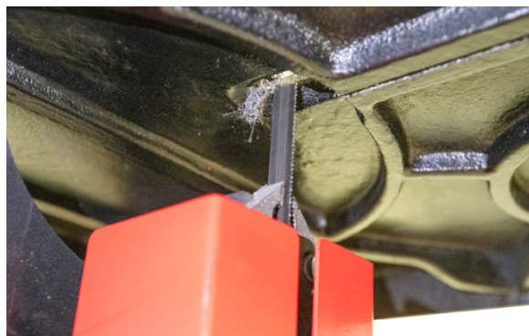
Figure 9-8 Lower Blade Guide
