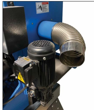
Figure 7-1: Dust Hood Outlet
