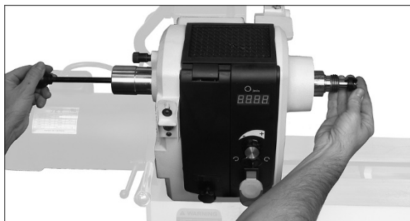
Figure 7-8: removing spur center
