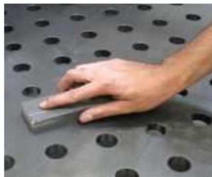
(4.5) wipe away slag with oil stone
