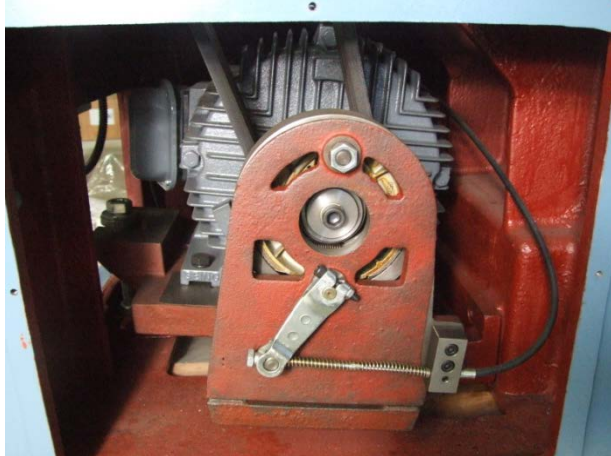
Figure 12 shows the cable and brake mechanism that is actuated by stepping on the brake pedal.
